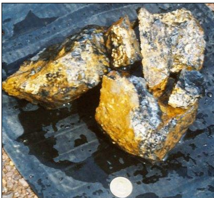
Figure 18. Gold in dark vein quartz from the supergene-enriched oxidized zone of the Lily gold mine. Approximately 60 oz gold are shown in the photograph. The gold was recovered in 1963 from an ore shoot that contained several other bonanza ore pockets. The gold shown was found at a depth of approximately 30 m below surface. The coin used for scale measures about 30mm in diameter.
